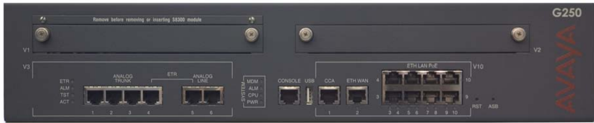
Figure 4: The G250 front panel ports and slots
