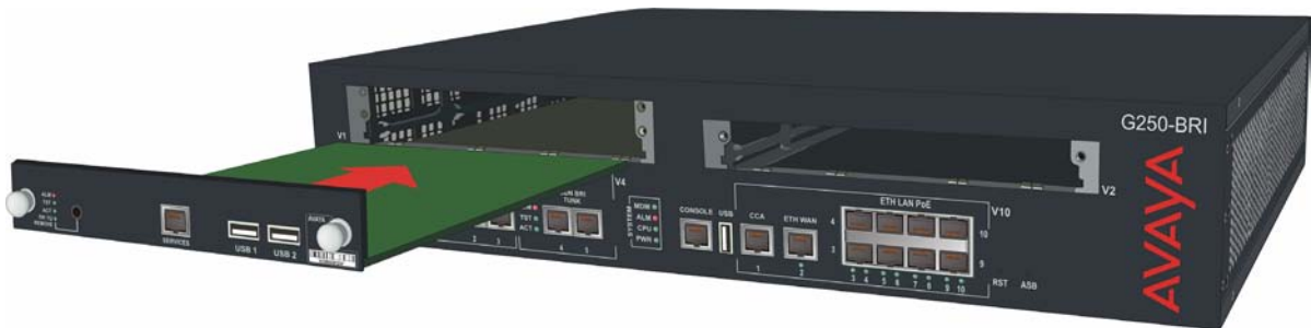
Figure 5: Inserting the S8300B media server module.
