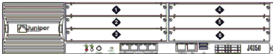
Figure 13: Slot numbers on the Juniper J4350 Services Router
