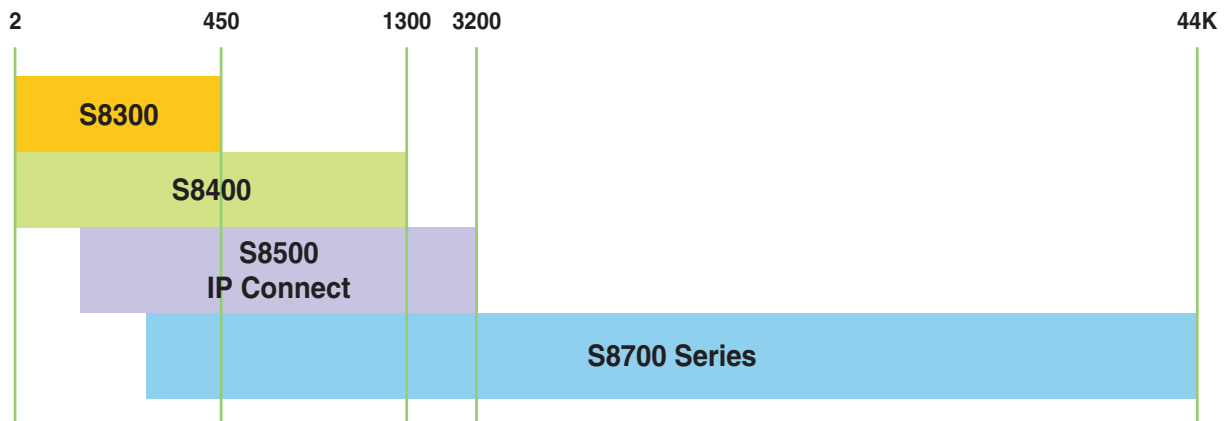
Figure 4: Avaya Application Solutions platforms port capacities
